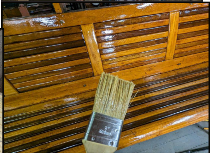
Above right: Car 1875's seat minutes after a fresh coat of varnish was applied.
