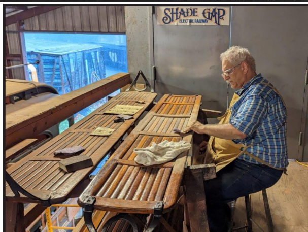
Bottom left: New volunteer Kevin Nolish sands a seat back for Open Car 1875.
