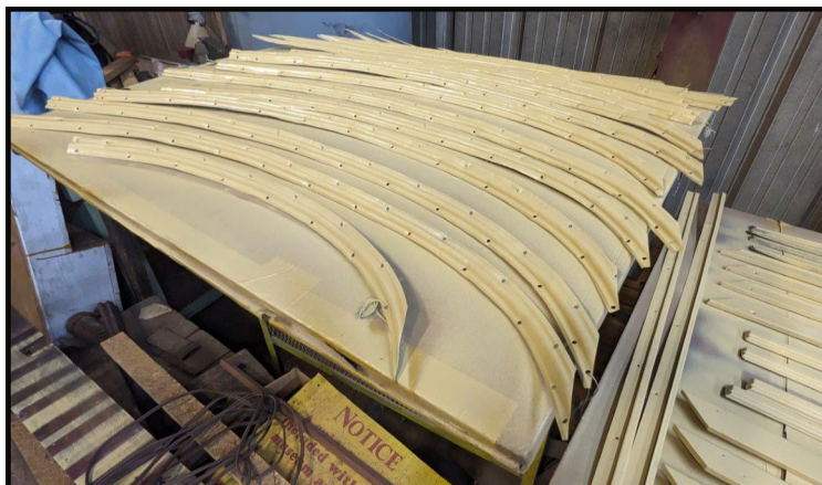
Above left: Car 315 trim pieces for the upper clerestory painted and ready to be installed.
