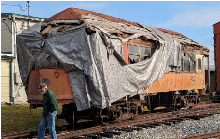
Top left: Volunteers assess the situation on how to best remove the subroof from the top of York 162 in November 2024 to prepare the car for moving to the museum. Top right: Car 162 before it was moved to Rockhill Trolley Museum in January 2025. Bottom photos: Car 162 is looking much more like a trolley after the roof was removed in one day.
